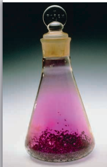
Iodine gas in a stoppered flask. Iodine is a crystalline solid at room temperature, but sublimates on heating to form a purple gas.
